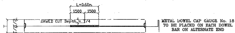
CONSTRUCTION JOINT SECTION
